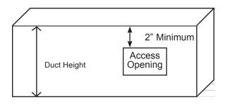
In order to use the minimum duct height, the door must be installed with it's longest dimension running horizontally along the length of the duct. If the minimum duct height is used, the top of the opening must be 2" from the top of the duct. For every inch over the minimum duct height, the opening can be lowered 1" from the top of the duct.
